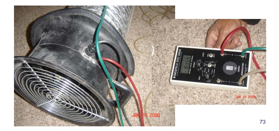
Connect a third hose to the Channel B Reference and to the plastic pressure tap on the duct blaster (green)
