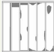
Compression or incomplete fill: <10% of area, compressed by <30% of intended thickness
