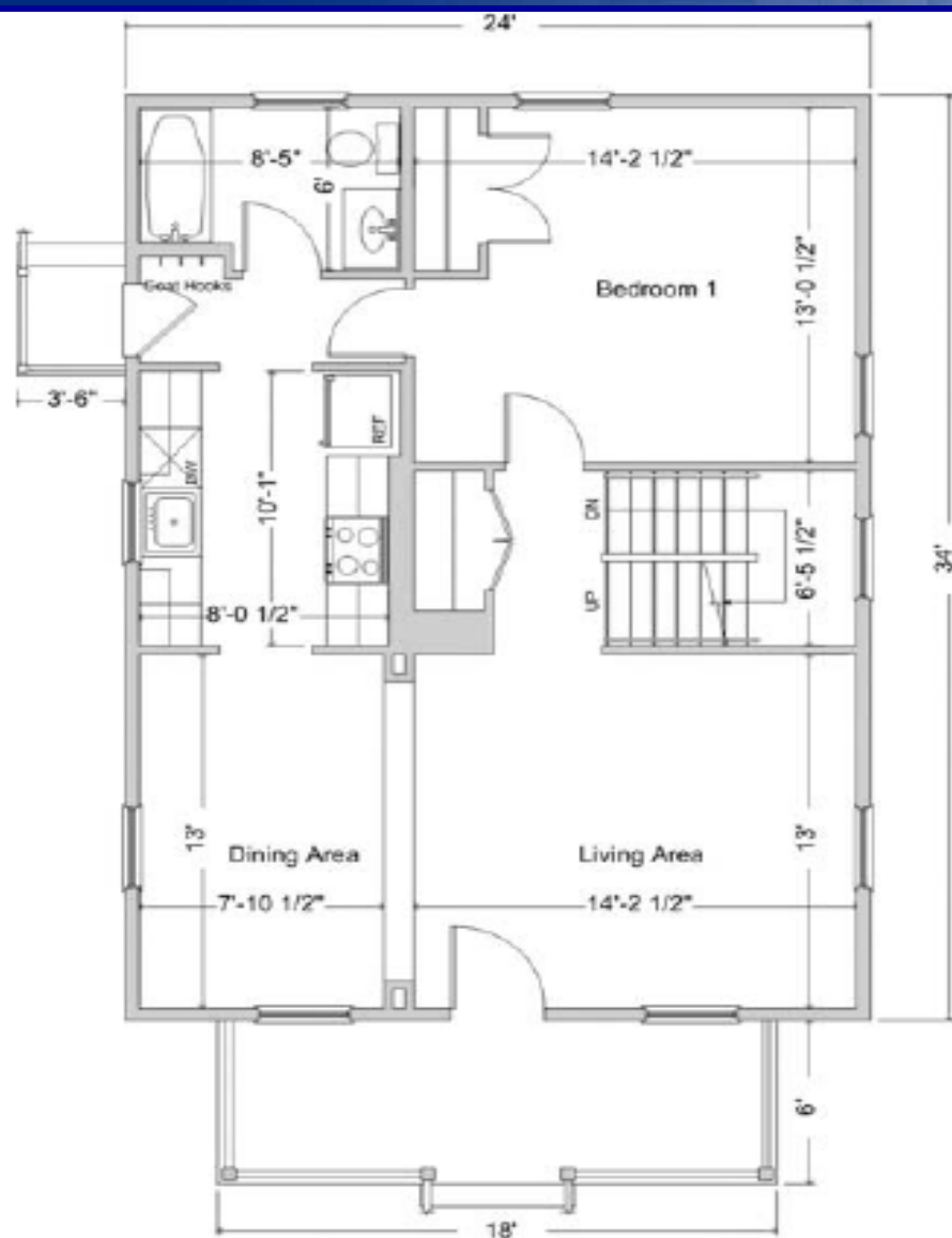
Figure 2: Mixed-Humid floor plans (Right: Ground Floor, Left: Second Floor, crawlspace not shown)
