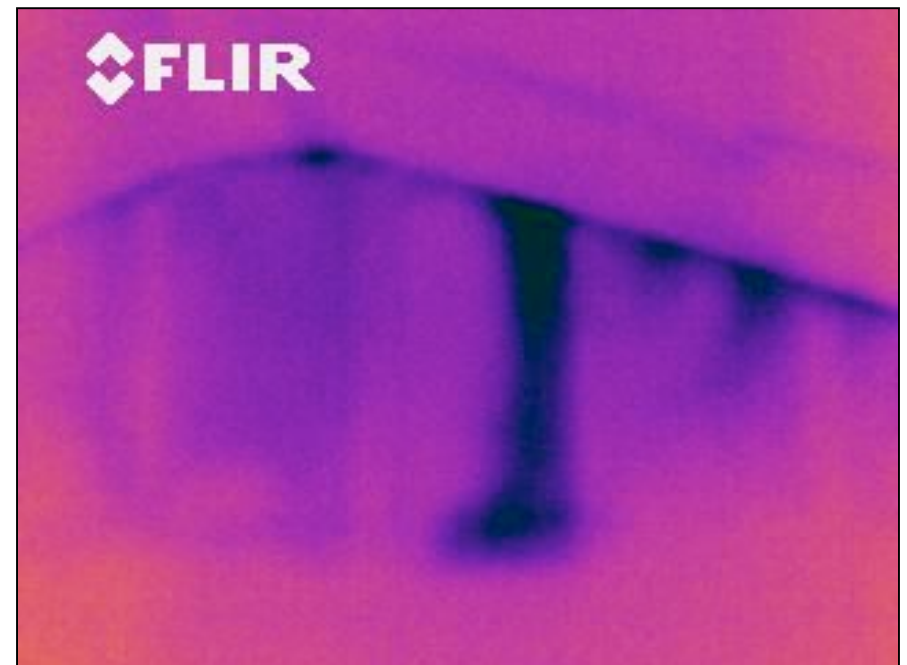
Small gable party wall showing batt falling off the back of wall
