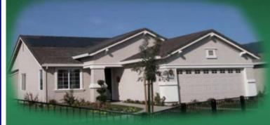
The "PowerHouse" is a high-performance house with an optional integrated photovoltaic roof shingle system. Generating nearly 6000 kWh annually, this more than offsets the anticipated annual electrical usage, creating a true "zero-net-electric" house.
