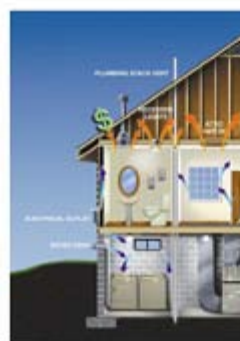
Diagram of Leaky Home: Leaks are often found at holes and plumbing, wiring, lighting, and doors.
