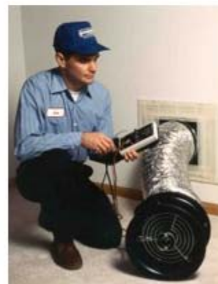
Photo of Man Conducting Duct Leakage Test
