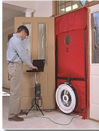
**Energy Raters use controlled airflow to estimate the amount of uncontrolled airflow.**
